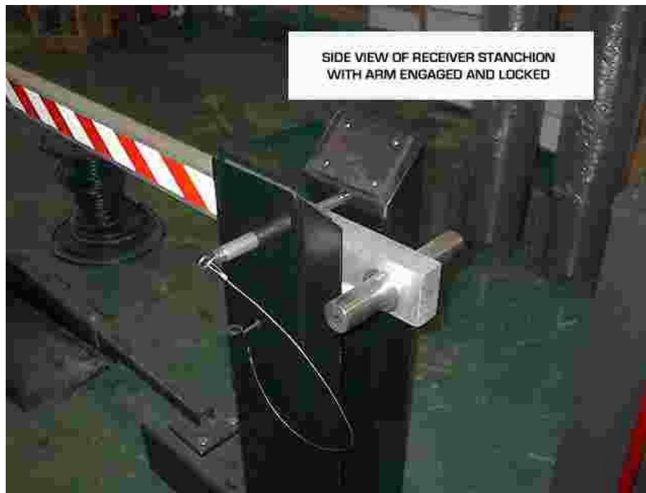
Figure 1-1: Receiver Post Stanchion and Security Latching Pin
