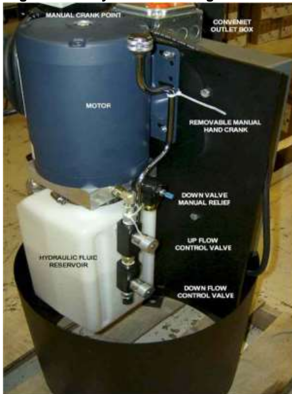
Figure 1-1c: Hydraulic Unit Right Side View
