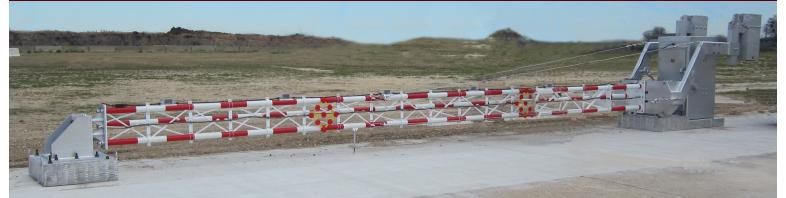
A VT-6802HDTR is a heavy-duty, vertically-operated, penetrationresistant, barrier system used to cover wide spans in locations that may experience harsh environmental conditions. Composed of an electrically driven vertical operator driving a cable reinforced tri-rail arm, the barrier system uses cable anchorages to provide the stopping force need to be certified to MASH TL-2.
