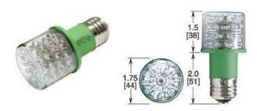
**GENERAL CONSTRUCTION:** Lamp shall consist of a 4-tiered array of 48 individual LEDs in an optically clear elastomer medium. In the event of failure of one or more individual LEDs, remaining LEDs shall continue to operate. Entire assembly shall be neatly potted into a molded Rynite FR350 stem fitted with a standard medium screw Edison base. Lamp head shall be filled with an optically clear silicon gel.
