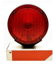
**Typical Use Notes**: This is typically used on warning gate arms or vertical barrier arms, spaced 4' to 7' apart. Often, the end light is wired to burn continuously and the remaining lights flash alternately (see separate specs for arm light flasher). Lights are normally controlled by the limit switch (see separate specification) to be off when the gate is open to traffic and on at all other times.
