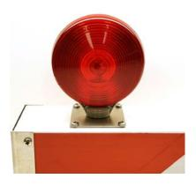
Typical Use Notes: This light is typically used on warning gate arms or vertical barrier arms, spaced 4' to 7' apart. Often, the end light is wired to burn continuously and the remaining lights flash alternately (see separate specs for arm light flasher). Lights are normally controlled by the limit switch (see separate specification) to be off when the gate is open to traffic and on at all other times.
